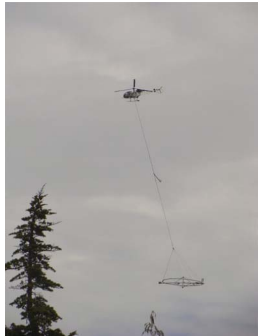
A helicopter doing an airborne electro-magnetic survey
