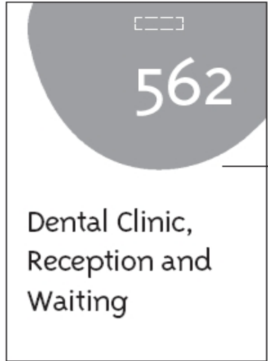
O Room ID interior 25mm tactile number; braille 14mm (cap) non-tactile legend
